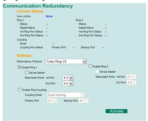
**NOTE** When using a dual-ring architecture, users must complete configuration for both Ring 1 and Ring 2. The status of both rings will appear under **Current Status**.
